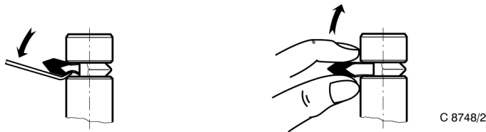
Figure 2 Removing KNORR K-rings (outer ring) Draw the ring out of its groove by the special hook, and pull it entirely off by hand. Or: Draw the ring taut between thumb and index finger. The ring emerges from its groove at the opposite side. Pull off the ring by hand.
