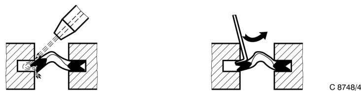
Figure 4 Removing KNORR K-rings (inner ring) Blow a jet of compressed air slantingly into the groove. The KNORR K-ring is blown up behind its sealing lips and jumps out of the groove. Or: Slip the special hook into the groove above the KNORR K-ring. Push out the KNORR K-ring by applying light pressure downwards.
