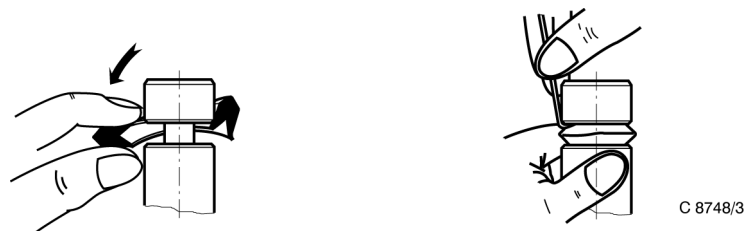
Figure 3 Installing KNORR K-rings (outer ring) Draw the thinly greased KNORR K-ring over the piston. Stretch the ring to one side and slip by hand into the groove with the sealing lips first. Repeat the procedure around the full circumference until the entire ring is seated in its groove. Run the special hook round between the KNORR K-ring and the groove wall.
